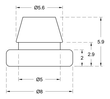
MOUNTING HOLE Ø 4.5-5.0 THICKNESS: 0.8-1.0
