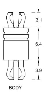
HOLE IN PCB Ø 3.2 THICKNESS 0.9
