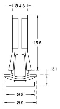
HOLE IN CHASSIS: Ø 4.8mm CHASSIS THICKNESS: 1.6mm
