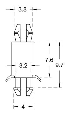
HOLE IN PCB Ø 3.3 THICKNESS :1.6-1.7
