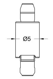
HOLE IN PCB Ø 3.2 THICKNESS :1.7-2.1
