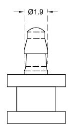
HOLE IN P.C.B: Ø 2.0 THICKNESS 1.6
