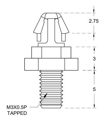
MOUNTING HOLE Ø 3.5 CHASSIS THICKNESS 1.6
